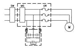
Figure 2: For existing motor installations Capacitors are connected to line side of thermal-overload relay. In this case the overload relay does not have to be resized
